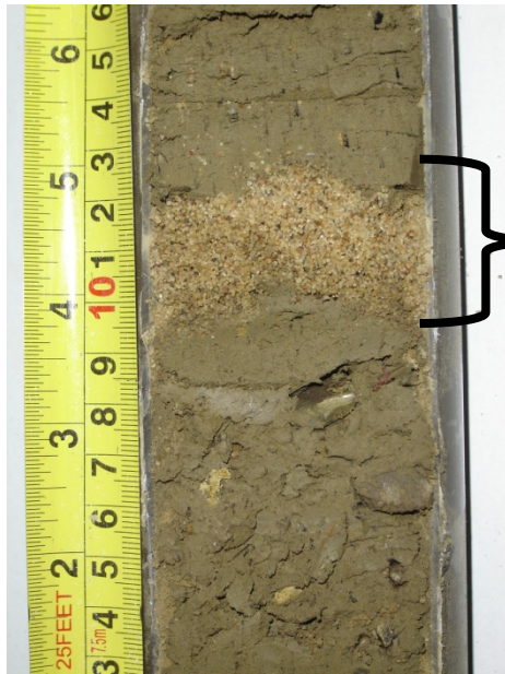
Sand-filled permeable treatment pathway in clay (2 cm thick)
