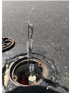
Thick membrane sampler plus duplicate being deployed in a soil probe
